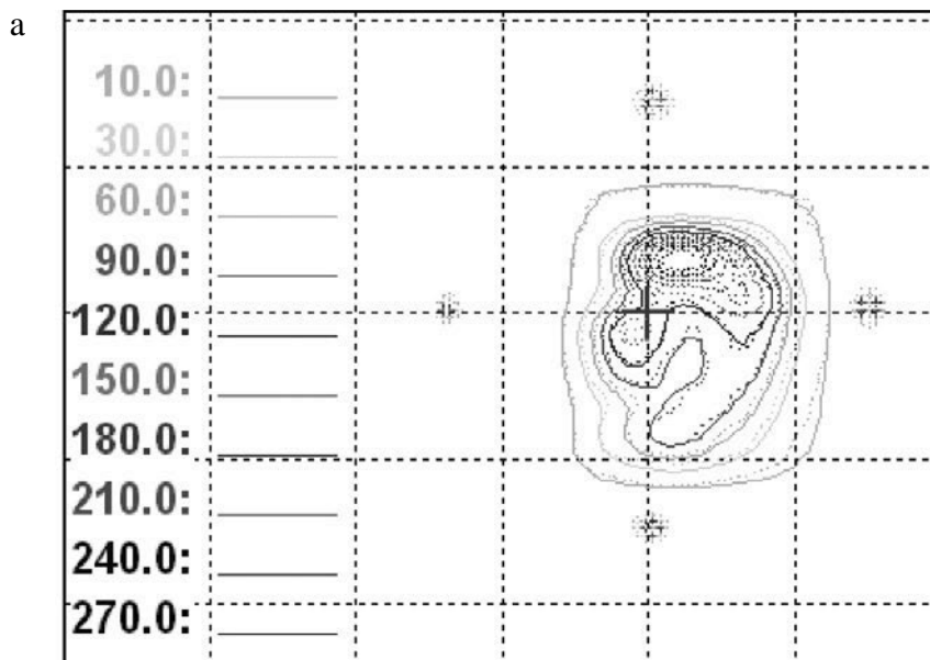
LSPO Dose Overlay. (Dotted Line - Film, Solid Line - TPS)
