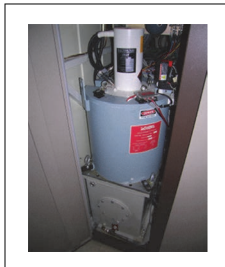
Figure 9.16 A klystron inside the gantry stand of a high-energy standing wave linac. The tank of insulating oil can be seen at the bottom.
