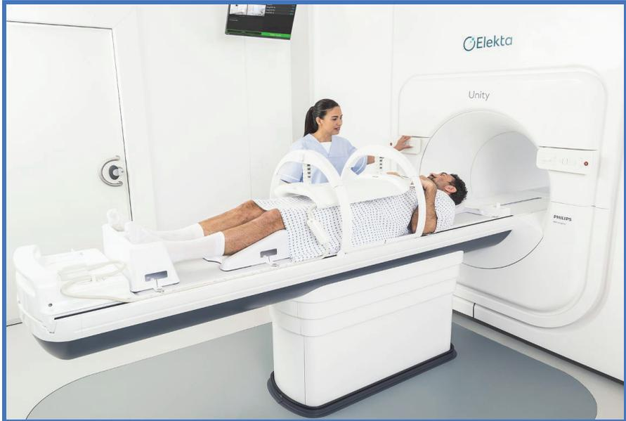
**Figure 1.27** Elekta Unity MRI-linac combining a 7-MV linac with 1.5-T MRI for image guidance. An extra mounted body coil is shown which is employed in combination with a gantry-mounted body coil to enhance image quality. (Image courtesy of Elekta.)
